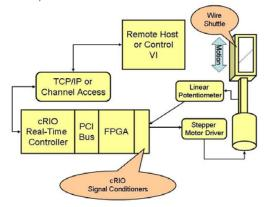
Figure 3. Wire Scanner Control Architecture
