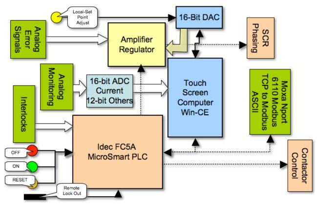
Figure 3 . Interaction between control elements in the controller
