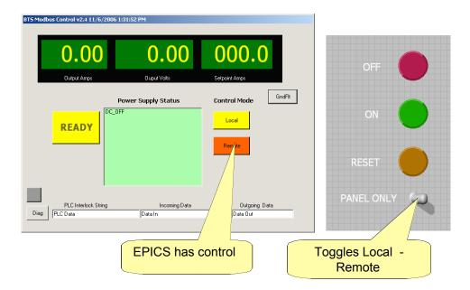
Figure 2 Display layout and relationship to physical buttons.
