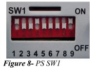
SW1-1 sets Remote Analog Programming, SW1-4 sets the output monitoring range to 0-10V, and SW1-9 sets the rear panel enable control.
