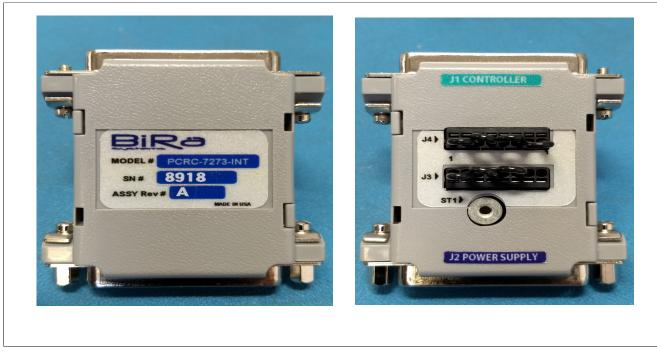
Figure 5- Interface Adapter (Front/Rear)
