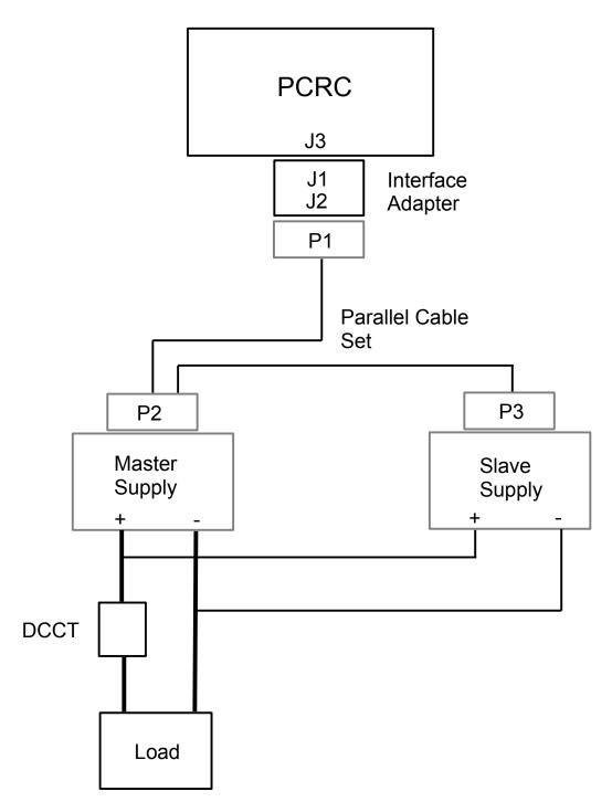
Figure 10- Parallel Setup Configuration Diagram
