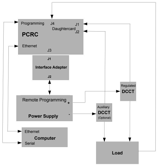
Figure 4- Typical System Setup Diagram
