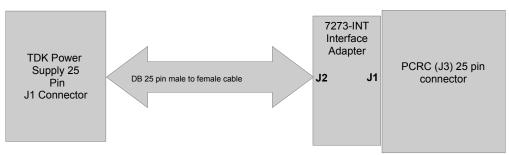
Figure 6- Interface Adapter Connection Diagram
