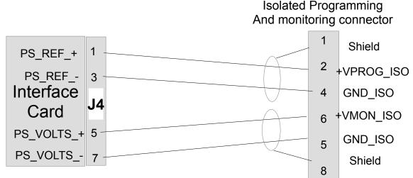
Figure 7- Isolated Analog Connections
