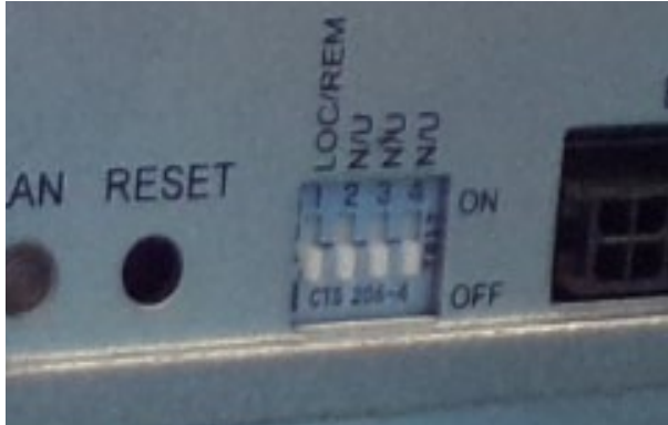
Figure 7- Rear Panel 4 position DIP Switch
