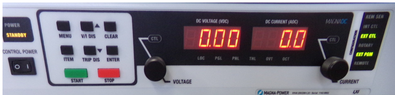
Figure 8- Magna Power Front Panel set for External control
