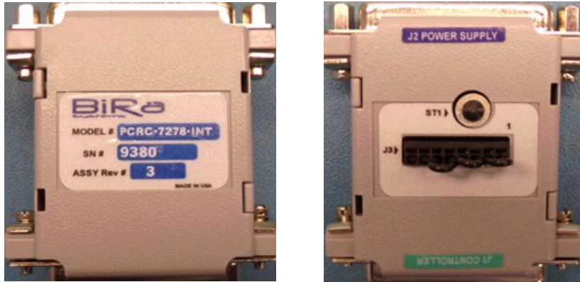
Figure 5- PCRC 7278-INT Interface Adapter (Front/Rear)
