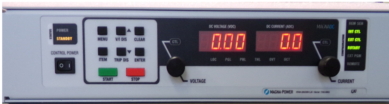
Figure 7- Magna Power Front Panel set for Local or Internal control
