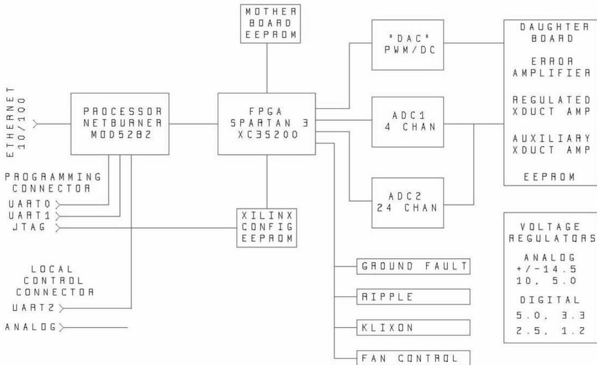
Figure 2: internal structure of the EPSC
