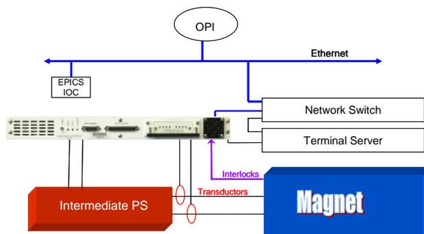
Figure 1: The Intermediate PS Architecture
