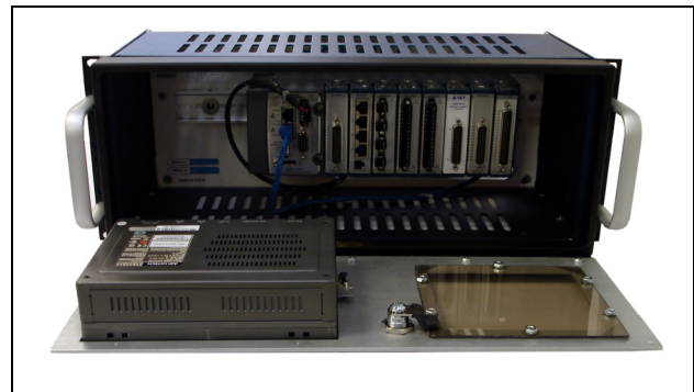
Figure 2: Wire Scanner System BiRIO Chassis.
